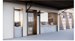
EXTERNAL GLAZING FILM SIGNAGE IN GOLD FOL, FINISH: TEXT: LUNE LOGO. OPENING: HOLE TOTAL WIDTH TO BE 450mm. EVERYTHING ELSE IN PROPORTION TO TEXT WIDTH.
